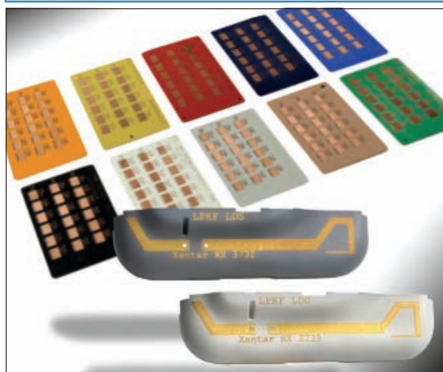
▲ Fig. 2 The colorful world of LDS using Xantar LDS from Mitsubishi Engineering Plastics (Source: MEP).
